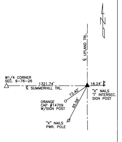
DISTANCES PLUMB CHAINED NW CORNER NE1/4 SW1/4 SECTION 9-76-26
