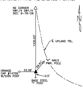
DISTANCES PLUMB CHAINED SE CORNER NW1/4 SW1/4 SECTION 9-76-26
