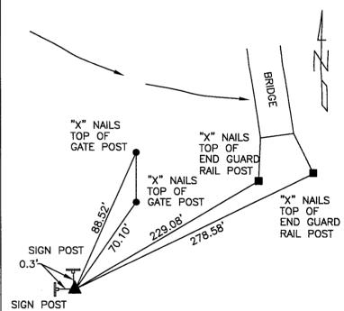
DISTANCES PLUMB CHAINED CORNER SW1/4 NW1/4 SECTION 9-76-26
