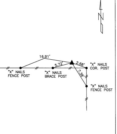
DISTANCES PLUMB CHAINED NW CORNER NE1/4 NE1/4 SECTION 8-76-26
