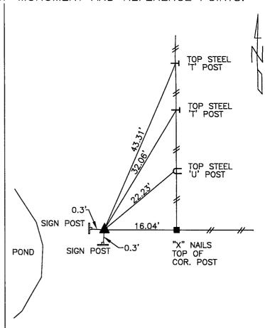
DISTANCES PLUMB CHAINED NW CORNER SE1/4 NE1/4 SECTION 8-76-26
