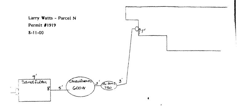
Sand filter - wood frame lined with garden felt on inside four (4) foot deep
