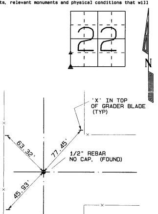
NW CORNER S1/2 SW1/4 SECTION 22-77-27 FOUND 1/2" REBAR IN CENTER OF INTERSECTION.
