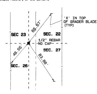
SW CORNER SECTION 22-77-27 FOUND 1/2" REBAR 8' WEST OF CENTER OF ROAD.
