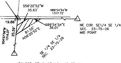
SW COR. SE1/4 SE 1/4 23-75-26 SET 1/2" REBAR YPC #15219 @FENCE COR. IN LINE W/SW & S1/4 COR.
