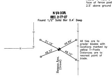
Set "x" nails in W face of fence post 1.2' above ground Set "x" nails SW face of corner fence post 0.5' above ground Set "x" nails in S face of fence post 12.95 1.3' above ground
