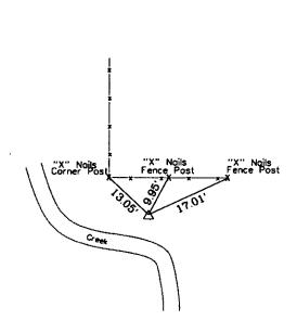
South 1/16 Cor. Section 7-76-27 Set 1/2" Rebar With Yellow Cap # 14674
