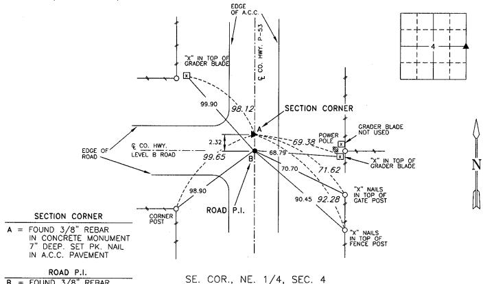
B = FOUND 3/8" REBAR 6" DEEP. SET PK. NAIL IN A.C.C. PAVEMENT
