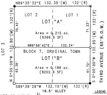
NOTE: This division of Lots 1 & 2 follows the center wall of an attached duplex which was under construction at the time of this survey.
