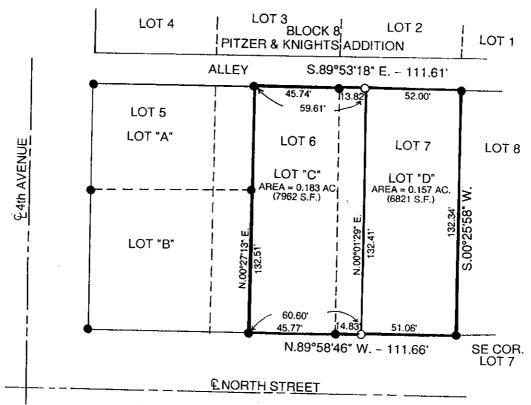
NOTE: This division of Lot 7 and a portion of Lot 6 follows the center wall of an attached duplex which was constructed at the time at the survey.
