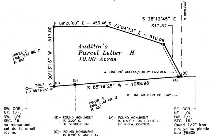
MEASURED DISTANCE/BEARING - (M) RECORDED DISTANCE/BEARING - (R)
