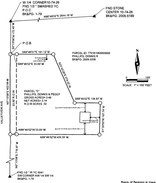
Basis of Bearing is Iowa State Plane Coordinate System South Zone.
