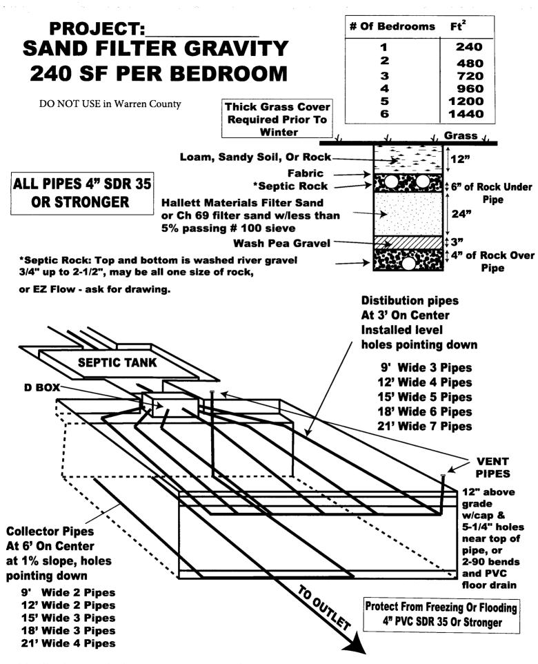
Distribution and Collector pipes may use 4" PVC lateral pipes as noted in Chapter 69. 9(4)d or 4" PVC with 1/2" holes spaced at 24", holes pointing down.
