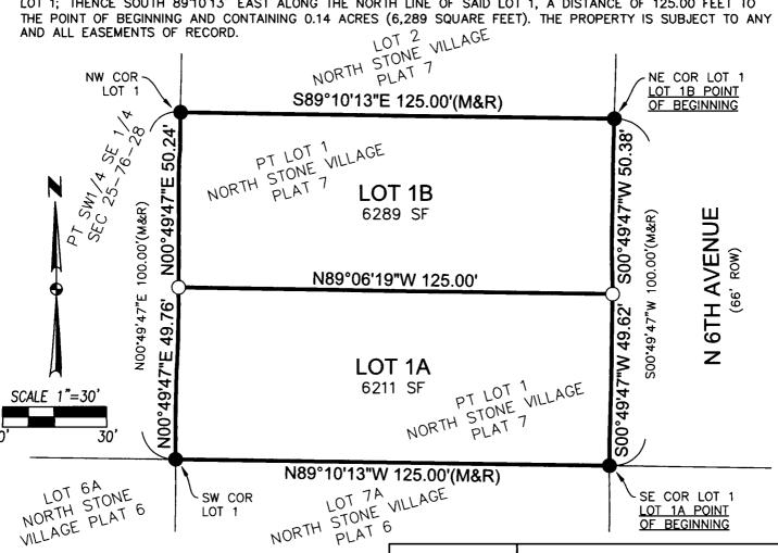
LEGEND **FOUND** 51004 SET SECTION CORNER AS NOTED Δ 1/2" REBAR, YELLOW PLASTIC CAP#15980 (UNLESS OTHERWISE NOTED) 0 MEASURED BEARING & DISTANCE М RECORDED BEARING & DISTANCE AWOL R DEEDED BEARING & DISTANCE D CENTERLINE SECTION LINE
