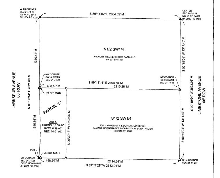
Basis of Bearing is Iowa State Plane Coordinate System South Zone
