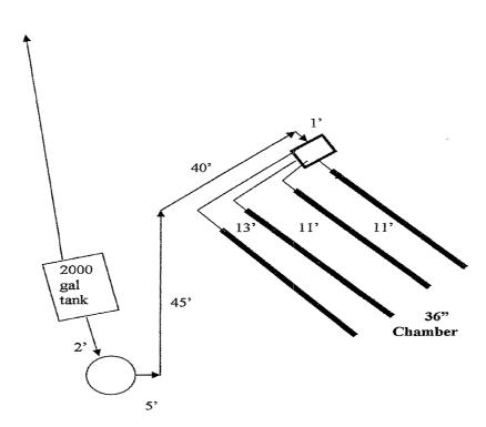
Used perc test from Vance & Hochstettler dated 6-24-04  $\,$  500' 5 @ 100. Used 36" Chamber and reduced 25%
